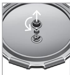
Unscrew the valve body (9A) anticlockwise and remove it from the lid. Clean thoroughly.
