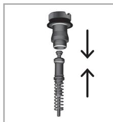
Reassemble the valve and place it back on the lid.
